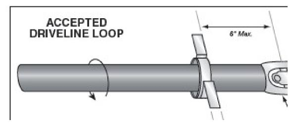
DRIVESHAFT TUBE DEFINITION: Driveshaft must be covered by a 360-degree round, oval, or tapered tube, covering the front U-joint and extending rearward a minimum 12 inches. Minimum thickness of tube is .050-inch steel or titanium. Driveshaft tube must utilize a minimum of four attachment points to the chassis, using either minimum 5/16 SAE Grade 8 bolts, welded, or 1/4-inch push/pull pins. Two-piece tube assembly permitted with a minimum of six 3/8-inch SAE Grade 8 bolts.
