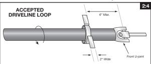
For all full-bodied and open-bodied cars running between 7.50 (\*4.50) and 13.99 (\*8.59) in place of a crossmember located behind but within 6 inches of the center of the front universal joint: A front driveshaft loop is required on all cars, except vehicles running 11.49 (\*7.35) seconds or slower equipped with street tires. See Class Requirements.
