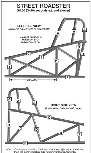
Mild steel construction requires .118" minimum wall thickness. Lower frame of square tubing minimum is 2" x 2" x .058".
