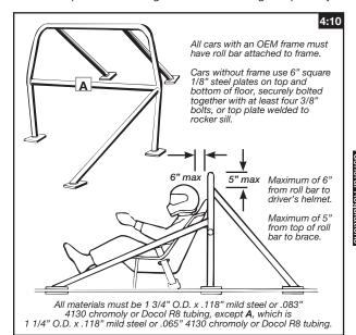
Any grinding of welds prohibited. See illustration. Roll bar must be padded anywhere driver's helmet may contact it while in driving position. Adequate padding must have minimum 1/4-inch compression or meet SFI Spec 45.1. All cars running 9.99 (\*6.39) or quicker, SFI Spec 45.1 mandatory.
